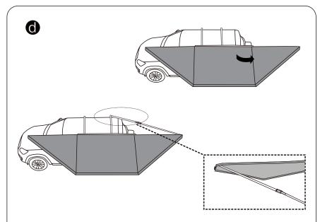
Whilst holding the awning poles and the canvas at the front, begin to walk in an arc towards the rear of the vehicle allowing the awning to rotate around the rear pivot. Once the first triangular section of canvas is tight and continue to pull back and pull out a rope and tie it to the top of the in.
